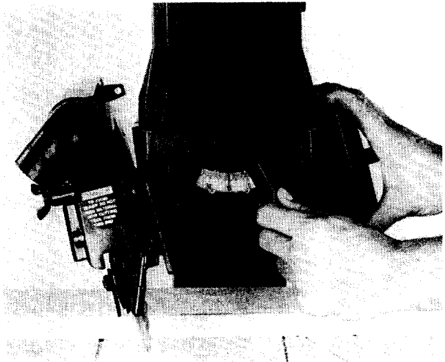
Fig. 28 - Bevel Lock - Unlocked
