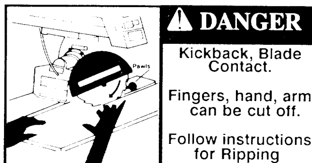
Fig. 101 - Kickback, Blade Contact Safety Sign
