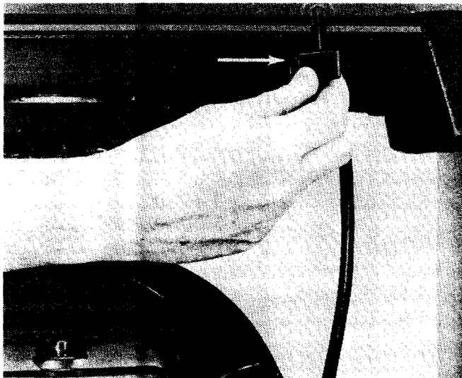
Fig. 92 - Locked Position for Rip Lock
