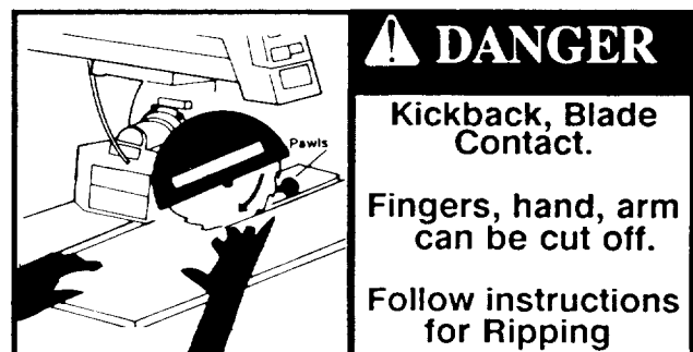
Fig. 3 Blade Contact Safety Sign
