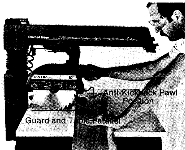
Fig. 100 Crosscut Blade Guard and Body Position
