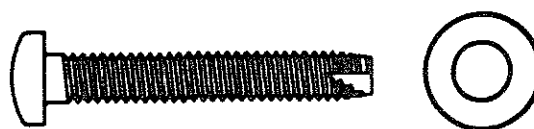
Fig. 81 - Mounting Screw and Washer
