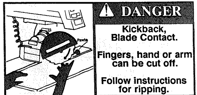
Fig. 151 Kickback, Blade Contact Safety Sign
