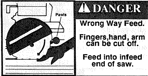
Fig. 4 Wrong Way Feed Safety Sign
