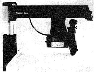
Fig. 97 Out-Rip Saw Position (Infeed End)
