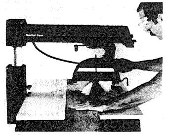
Fig. 86 Blade Distance to Complete Crosscut
