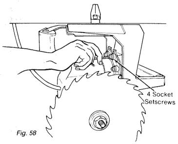
10. Hold the square in place and move the *motor* slowly until the square is flush with the *blade*.
