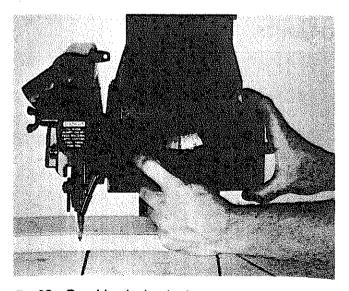
Fig. 29 - Bevel Lock - Locked
