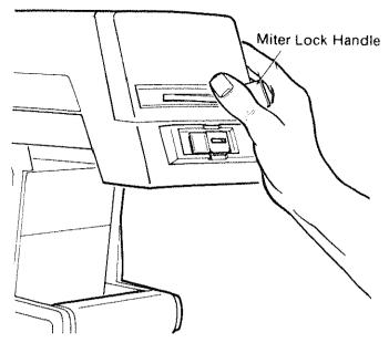
Fig. 128 - Miter Lock - Unlocked
