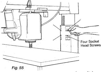
12. Use the top two screws to move the radial arm into line:
