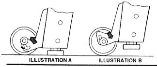
B. Never operate the tool with the casters in the down position—the entire weight of the tool must be supported by the levelers when operating the saw, jointer or other tool.
