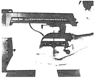
Fig. 92 Distance Needed to Complete Crosscut
