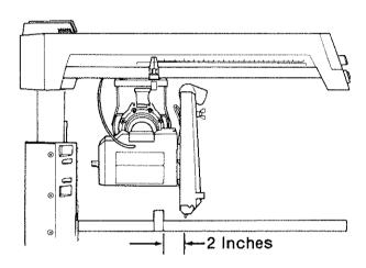
Fig. 78- Out-Rip Saw Position (Infeed End)
