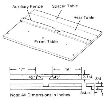
Fig. 114 Auxiliary Fence for Edging
