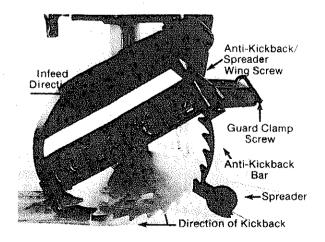
Fig. 103 Blade Guard Position for Ripping
