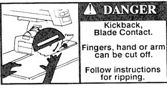
Fig. 98 Kickback, Blade Contact Safety Sign
