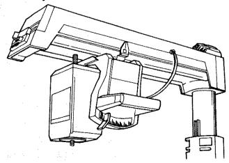
Fig. 108 Arbor Shaft Position When Using Accessory Shaft
