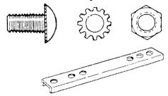
Fig. 23A - Bolt, External Lockwasher, Hex Nut, U-Channel
