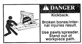
Fig. 99 Kickback, Thrown Workpiece Safety Sign
