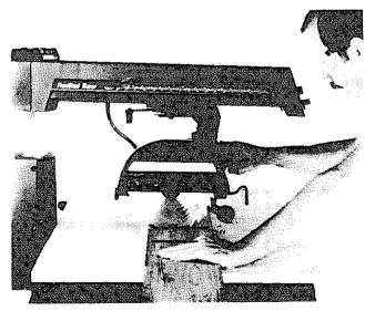
Fig. 93 Hand Placement for Crosscuts
