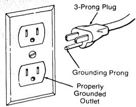
Fig. 79 - Plug for Less Than 150V
