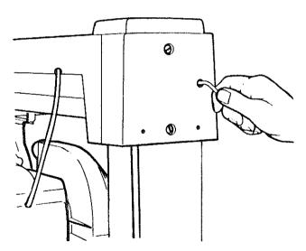
Fig. 129 - Location of Hex Socket Cap Screw
