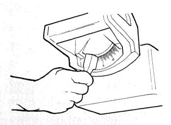
Fig. 122 - Bevel Lock - Locked
