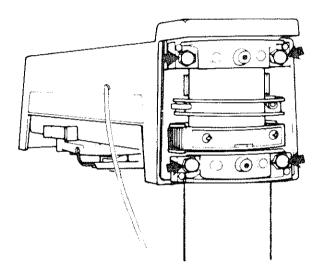
Fig. 125 - Location of Hex Head Tapping Screws
